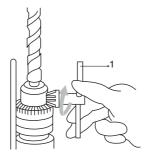
To install the bit, place it in the chuck as far as it will go. Tighten the chuck by hand. Place the chuck key in each of the three holes and tighten clockwise. Be sure to tighten all three chuck holes evenly. To remove the bit, turn the chuck key counterclockwise in just one hole, then loosen the chuck by hand. After using the chuck key, be sure to return to the original position.
