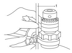
The depth gauge is convenient for drilling holes of uniform depth. Loosen the auxiliary handle and adjust the depth gauge to the desired depth. After adjusting, tighten the auxiliary handle.
