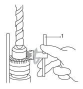
To install the bit, place it in the chuck as far as it will go. Tighten the chuck by hand. Place the chuck key in each of the three holes and tighten clockwise. Be sure to tighten all three chuck holes evenly. To remove the bit, turn the chuck key counterclockwise in just one hole, then loosen the chuck by hand. After using the chuck key, be sure to return to the
