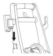
3) Installing the dust compartment into position
