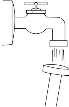
Clean the nozzle with the needle clean-out tool provided. Remove the spray wand from the gun. Remove any dirt from the nozzle hole and rinse.
