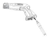
3. Connect the high-pressure hose to the water outlet
