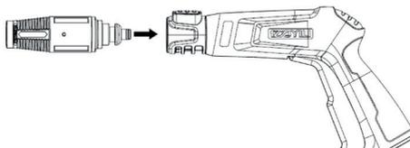
2. Connect the high pressure hose to the trigger gun. Connect the sliver end of the high-pressure hose to the trigger gun and twist the nut as indicated to secure the connection.
