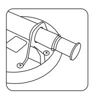
After cleaning the hand pressure pump, grease can be applied appropriately
