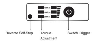
Torque adjustment, 200N.m / 300N.m / 350N.m indicator lights up when the switch trigger is pressed: Function keys 200N.m / 300N.m /350N.m switch; press forward and reverse switch keys.
