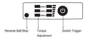
Torque adjustment, 230N.m / 180N.m / 100N.m indicator lights up when the switch trigger is pressed: Function keys 230N.m / 180N.m /100N.m switch; press forward and reverse switch keys.
