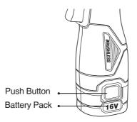
When removing the battery pack, press the button on the front side of the battery pack and pull the battery pack out of the tool at the same time. When installing the battery pack, align the tongue spring on the battery pack with the groove on the cover, and then push and slide it into place. Insert it fully into place until the battery pack is locked and clicks. If you can still see the red indicator on the upper side of the button after inserting it, it
