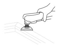
Apply a sanding paper on the workpiece.
