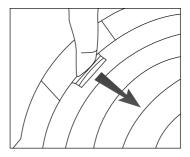
3. Connect the plastic hose end with the suction port, and turn it clockwise as the picture shows
