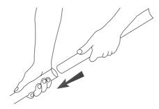
6. Connect the wet&dry brush with The plastic tube.
