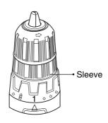
Turn the sleeve counterclockwise to open the chuck jaws. Place the bit in the chuck as far as it will go. Turn the sleeve clockwise to tighten the chuck. To remove the bit, turn the sleeve counterclockwise.
