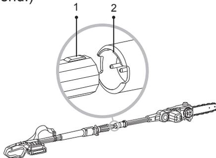
3- With the locking knob lock pole joints.
