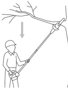
2- Never stand on a ladder or other type of unstable support while using the Pole saw. Always use both hands to operate the pole saw. Keep a firm, steady pressure on the pole saw while cutting but do not try to force the saw through the wood.
