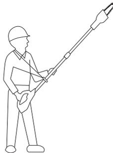
5- When ready to make a cut, press in trigger lockout and squeeze the trigger. This will turn the pole saw on. Releasing the trigger will turn the pole saw off.
