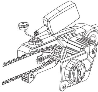
7- To insert the battery pack, groove along the handle and insert in the full position, until the Battery Release Button(18) bounces back to normal position again.
