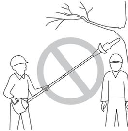
4- Do not use a pole saw near the cable, electric power, or telephone lines.
