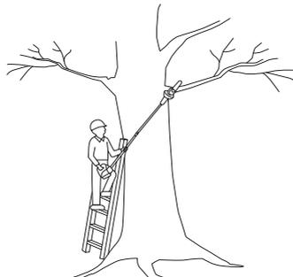
3- Keep other persons away from cutting the end of the pole saw and at a safe distance from the work area.
