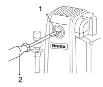
Both carbon brushes should be replaced at the same time. Use only identical carbon brushes. Use a screwdriver to remove the brush holder caps. Take out the worn carbon brushes, insert the new ones and secure the brush holder caps.
