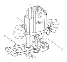
To install the straight guide, insert the guide bars into the holes in the plunge base. Adjust the distance between the bit and the straight guide. At the desired distance, tighten the wing bolts to secure the straight guide in place. When cutting, move the tool with the straight guide flush with the side of the workpiece.
