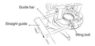
Install the straight guide on the guide holder with the wing nut. Insert the guide holder into the holes in the plunge base and tighten the wing bolts. To adjust the distance between the bit and the straight guide, loosen the wing nut. At the desired distance, tighten the wing nut to secure the straight guide in place.
