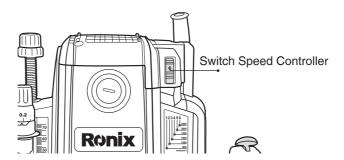
The tool speed can be changed by turning the speed adjusting dial to a given number setting from 1 to 6. Higher speed is obtained when the dial is turned in the direction of number 6. And lower speed is obtained when it is turned in the direction of number 1.
