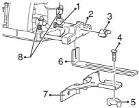
Install the straight guide on the guide holder with the wing nut. Insert the guide holder into the holes in the plunge base and tighten the wing bolts. To adjust the distance between the bit and the straight guide, loosen the wing nut. At the desired distance, tighten the wing nut to secure the straight guide in place.
