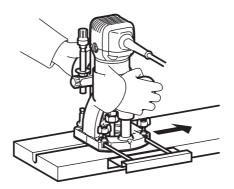
To install the straight guide, insert the guide bars into the holes in the plunge base. Adjust the distance between the bit and the straight guide. At the desired distance, tighten the wing bolts to secure the straight guide in place. When cutting, move the tool with the straight guide flush with the side of the workpiece.
