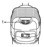
The tool speed can be changed by turning the speed adjusting dial to a given number setting from 1 to 6. Higher speed is obtained when the dial is turned in the direction of number 6. And lower speed is obtained when it is turned in the direction of number 1.
