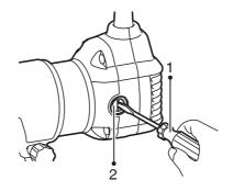
Both carbon brushes should be replaced at the same time. Use only identical carbon brushes. Use a screwdriver to remove the brush holder caps. Take out the worn carbon brushes, insert the new ones and secure the brush holder caps.
