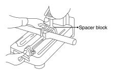
When the cut-off wheel has worn down considerably, use a spacer block of sturdy, non-flammable material behind the workpiece as shown in the figure. You can more efficiently utilize the worn wheel by using the mid point on the periphery of the wheel to cut the workpiece.
