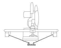
Long workpieces must be supported by blocks of non-flammable material on either side so that it will be level with the base top.
