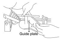
To change the cutting angle, loosen the two hex bolts which secure the guide plate. Move the guide plate to the desired angle (0-45) and tighten the hex bolts securely.
