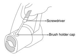
Use a screwdriver to remove the brush holder caps. Take out the worn carbon brushes, insert the new ones and secure the brush holder caps. To maintain product SFAETY and RELIABILITY, repairs, any other maintenance or adjustment should be performed by Makita Authorized or Factory Service Centers, always using Makita replacement parts.
