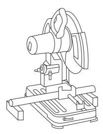
Press the switch trigger of the machine, it switches on, loose the trigger completely, the machine is under switch off condition. The machine switch can be locked if needing to make the machine runs continuously please press the locking button at the time of pressing the switch trigger completely, the machine will be under working condition. If need to release the locking, press the switch trigger again.
