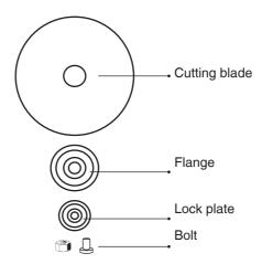
When the cutting wheel is wearing out, it can also be used economically and efficiently by adjusting the height of hexagonal bolts to control the cutting angle.
