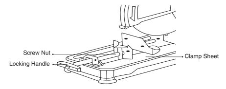
When cutting long object, put two nonflammable cushions under two ends of it, and make the object to keep in level with the pan base, ensure the supporting plain of the two cushions an the supporting plain of the base plate in a straight line.
