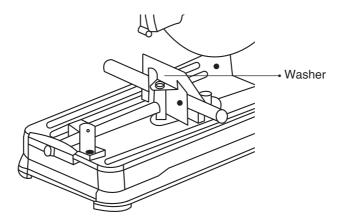
Only when cutting small object and the object can be fully clamping may the cushion be used in this manner.
