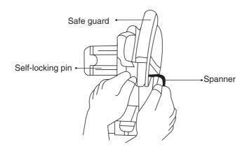
When disassemble the cutting wheel, firstly pull up the movable safety guard and press the self-locking pin to fix the cutting wheel, unscrew the hex bolt counterclockwise with wrench, and then take down the flangeand the cutting wheel.
