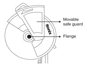
When assemble the cutting wheel, the steps are opposite to the abovesaid steps.
