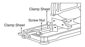
When the cutting wheel is worn out greatly, put a nonflammable hard cushion under the back of the work piece, thus it can use the middle edge of the cutting wheel to cut the object efficiently.
