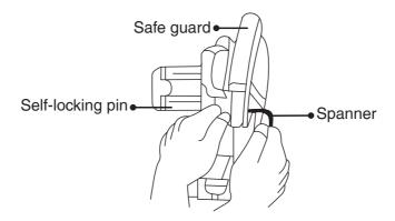
When disassemble the cutting wheel, firstly pull up the movable safety
