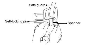
When disassemble the cutting wheel, firstly pull up the movable safety guard and press the self-locking pin to fix the cutting wheel, unscrew the hex bolt counterclockwise with wrench, and then take down the flangeand the cutting wheel.
