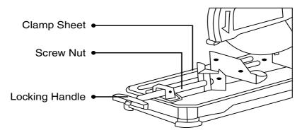
When the cutting wheel is worn out greatly, put a nonflammable hard cushion under the back of the work piece, thus it can use the middle edge of the cutting wheel to cut the object efficiently.
