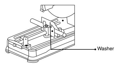
Only when cutting small object and the object can be fully clamping may the cushion be used in this manner.
