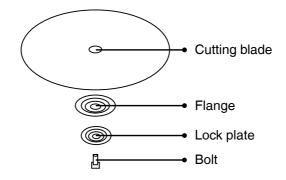
When the cutting wheel is wearing out, it can also be used economically and efficiently by adjusting the height of hexagonal bolts to control the cutting angle.
