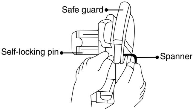
When disassemble the cutting wheel, firstly pull up the movable safety guard and press the self-locking pin to fix the cutting wheel, unscrew the hex bolt counterclockwise with wrench, and then take down the flange and the cutting wheel.
