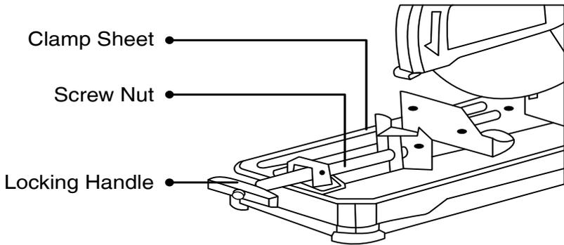
When the cutting wheel is worn out greatly, put a nonflammable hard cushion under the back of the work piece, thus it can use the middle edge of the cutting wheel to cut the object efficiently.
