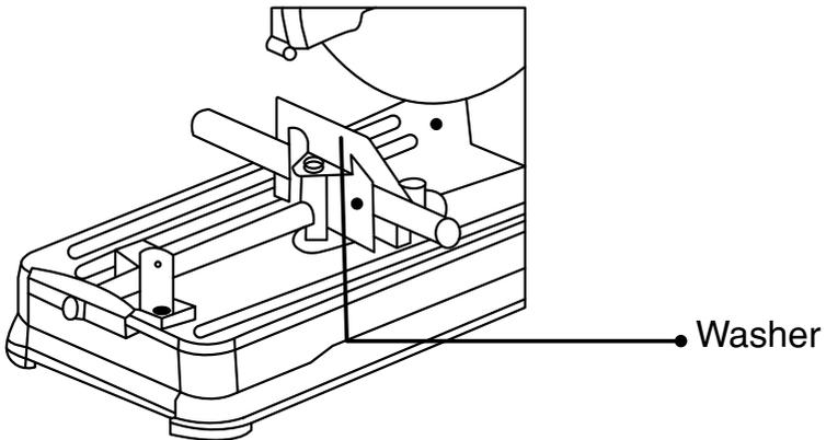
Only when cutting small object and the object can be fully clamping may the cushion be used in this manner.
