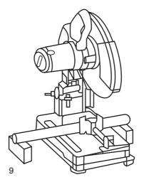
Press the switch trigger of the machine, it switches on; loose the trigger completely, the machine is under switch off condition. The machine switch can be locked if needing to make the machine runs
