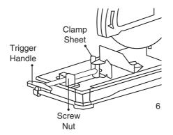
When the cutting wheel is worn out greatly, put a nonflammable hard cushion under the back of the work piece, thus it can use the middle edge of the cutting wheel to cut the object efficiently.
