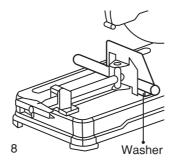
When cutting long object, put two nonflammable cushions under two ends of it, and make the object to keep in level with the pan base, ensure the supporting plain of the two cushions an the supporting plain of the base plate in a straight line.
