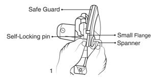
When disassemble the cutting wheel, firstly pull up the movable safety guard and press the self-locking pin to fix the cutting wheel; unscrew the hex bolt counterclockwise with wrench; and then take down the flange and the cutting wheel.
