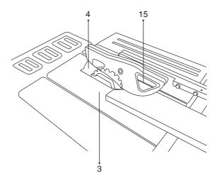
Longitudinal cutting (also known as slitting) is when you use the saw to cut along the grain of the wood.
