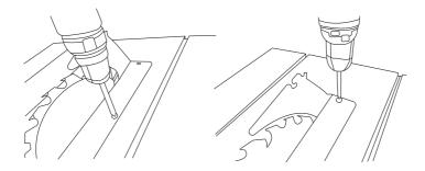
Step 2: Take out bench insert and find the nut fix riving knife.
