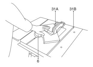
Slide the cross stop (6) into one of the grooves (31a/b) in the table and adjust to the required angle. If you also want to tilt the blade (3), use the groove (31a) which prevents your hand and the cross stop from making contact with the blade guard.
