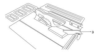
Be sure to use a push stick (9) when making longitudinal cuts in workpieces smaller than 120 mm in width.
