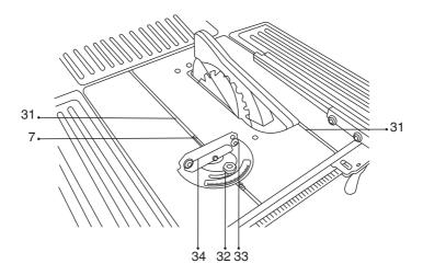
Push the transverse stop into a groove (31) of the saw bench.
