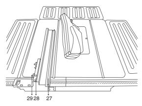
The stop rail of the rip fence (27) has two guide surfaces with different heights.
