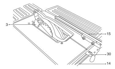
The rip fence (15) must be used for longitudinal cutting of wood parts. The rip fence (15) should be mounted on the right side of the saw blade (3). Set the rip fence (15) on top of the guide rail for rip fence (14).
