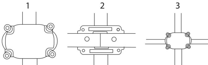
Refer to the pic 1~3, loose and take off the 4 screw and the upper clamp, Install the handle in to the middle clamp, then locked the screw
