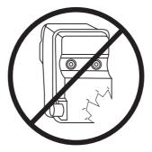
Bear in mind that: The exhaust fumes from the engine are hot and may contain sparks which can start a fire.
