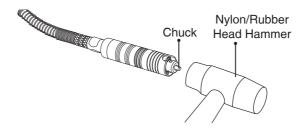
You can assemble tool like schematic pic as below
