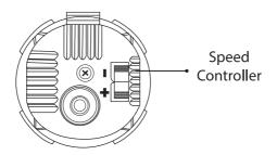
The number setting on the speed controller is equal to the tool speed.
