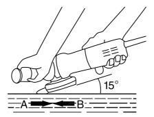
period with a new wheel, do not work the grinder in the B direction
