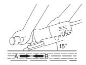
d)when using new disc,don't move the tools in B direction, otherwise the work piece maybe cut off. After the disc become round, then the tools could be moved in both A and B directions.
