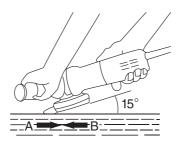
d)when using new disc,don't move the tools in B direction , otherwise the work piece maybe cut off. After the disc become round , then the tools could be moved in both A and B directions.
