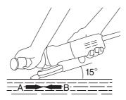
d)when using new disc,don't move the tools in B direction , otherwise the work piece maybe cut off. After the disc become round , then the tools could be moved in both A and B directions.
