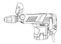
For low temperatures, the power tool reaches the full impact rate only after a certain time. This start-up time can be shortened by striking the chisel in the power tool against the floor one time.
