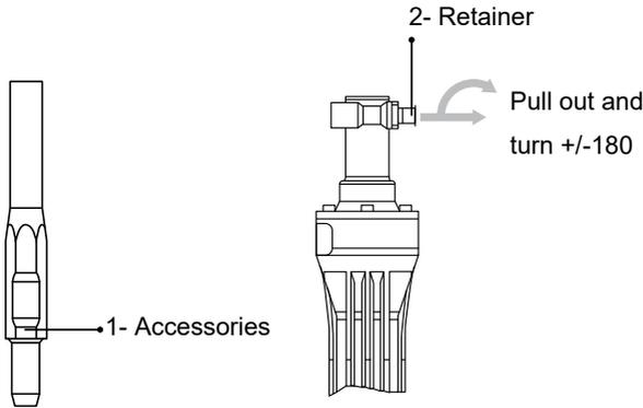
**! REMARKING:** When removing the accessory, such as a bull point, a cutter etc., follow above procedure in reverse order.
