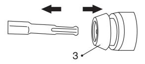
This electric hammer chisel does not have reverse direction, so always take care not to force the chisel in case the chisel bit gets stuck. Always make sure you keep the chisel going in and out to remove debris.
