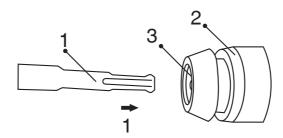
Put the bit into the hex housing and clamp the bit by turning the stop lever half a turn anti clockwise. This will lock the bit in place.
