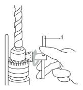
To install the bit, place it in the chuck as far as it will go. Tighten the
