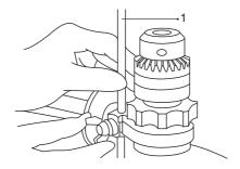
The depth gauge is convenient for drilling holes of uniform depth. Loosen the auxiliary handle and adjust the depth gauge to the desired depth. After adjusting, tighten the auxiliary handle.
