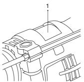
1- Knob for drilling/hammer drilling
