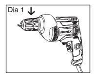
Turn chuckkey clockwiseto tighten
