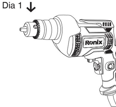
Turn chuckkey clockwiseto tighten
