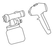
3) Clean the sprayer. Unscrew the container. Empty any remaining coating material back into the material tin. Use only solvents with a flashpoint over 38°C.
