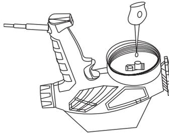
This will lubricate the piston and cylinder.
