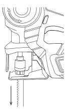
4. Pull on the blade to ensure it is properly secured.
