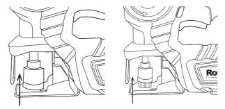
2. Blade can be installed with the teeth facing forward or backward to suit the application. Insert the T-shank into the blade holder.
