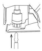
3. Release the quick release blade clamp.
