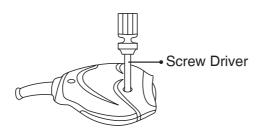
Take away the old brush, put on the new carbon brush and brush holder, fix on the carbon brush line and the stator line together.
